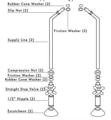
It is always suggested to apply plumber's tape to any threads before installation
