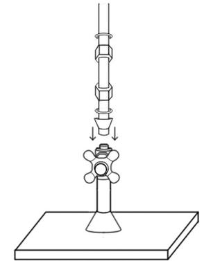
4. On the opposite end of the supply line, take a rubber cone washer and place it on the supply line with the flat side against the lip in the lines. Slide the slip nut and friction washer that you put on the pipe in step 3, up to the top of the lines. Tighten the nut to the faucet through the mouting holes of the tub.
