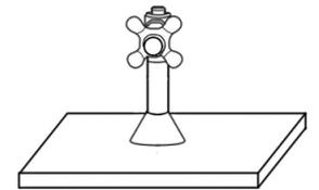
3. Take a friction washer and slip nut and slide them onto a supply line. The slip nut needs to be upside down when placing it on the supply line for later steps.
