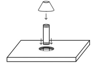
2. Once the nipple is tightened down, thread the straight stop valve onto the nipple. The handle on the valve should be facing away from the tub for easy access. On top of the valve will be a compression nut, friction washer, and rubber cone washer. Take these off for the next step.
