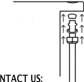
5. Repeat all the steps for the second water line and once fully installed, turn on the water to test for leaks.
